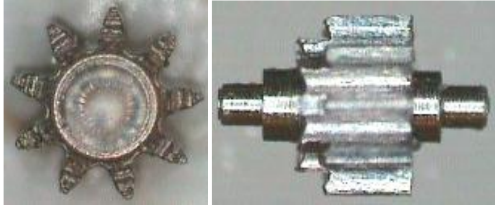
Fig. 2-25: The magnified reduction pinion sample machined by our machine
