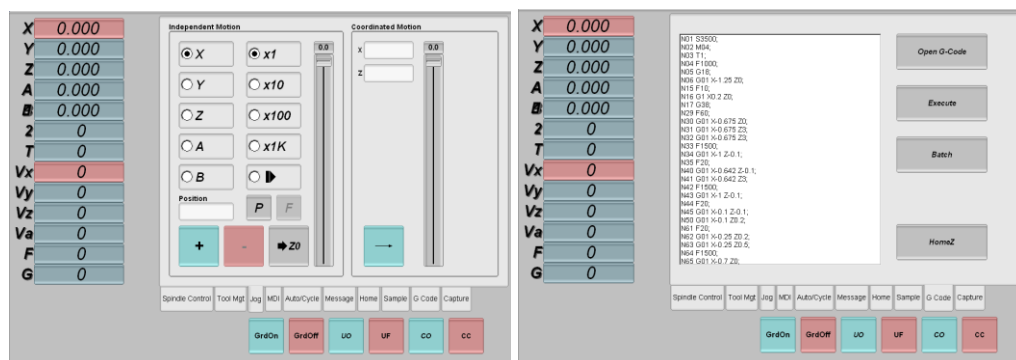
Fig. 2-14: Jog motion and G code interface
