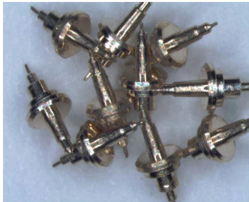
Fig. 2-20: Balance staff samples machined by the system
