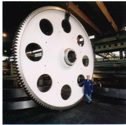
Fig. 1-13: Gear with diameter of 5m made by gear hobbing [28]
