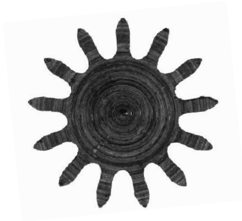
Fig. 3-24: The magnified sample gear machined by our machine
